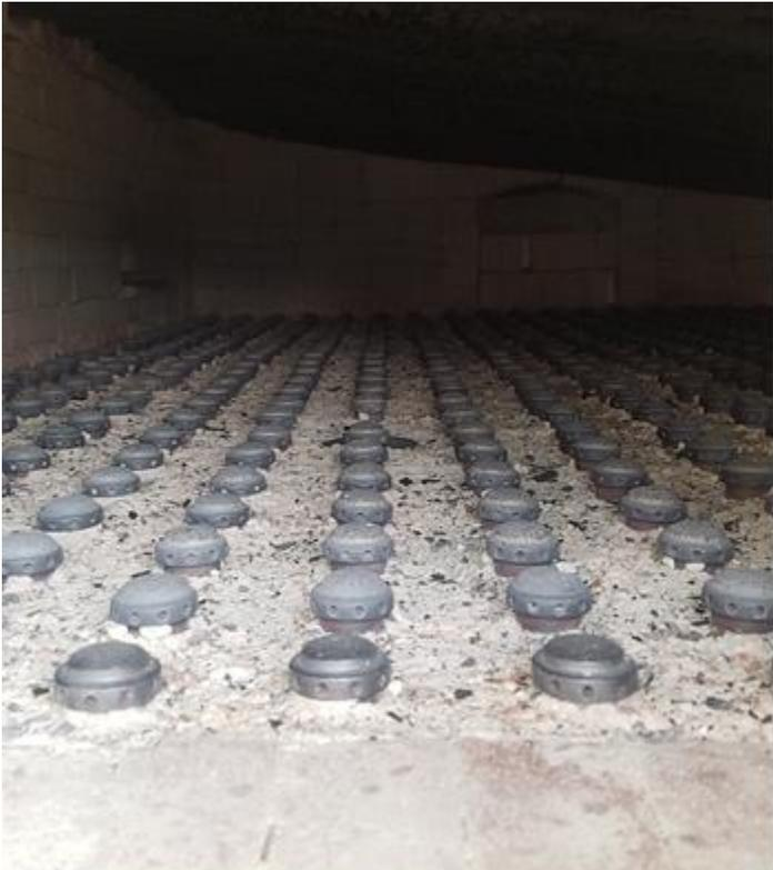
**Figure 3: Feeding mechanism of a reciprocating grate bio-mass boiler (feeding corn cob)**
