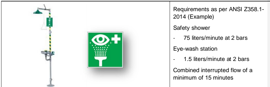
Figure 12 – Safety shower/emergency eye wash station
