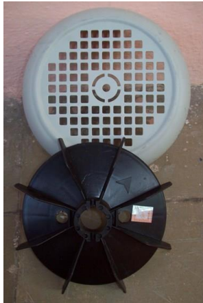
Use of fans with fan covers for engine cooling
