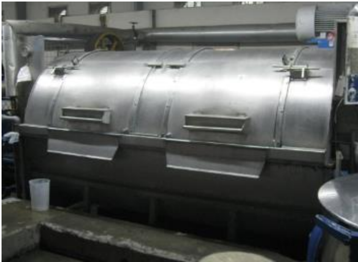
Horizontal cage industrial washing machine at a factory in Thai Binh
