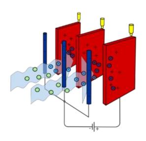
Electrostatic precipitation in combination with heat exchangers or scrubbers is successfully applied in the treatment of fumes emitted from the stenters where the fabric is submitted to thermofixation.
