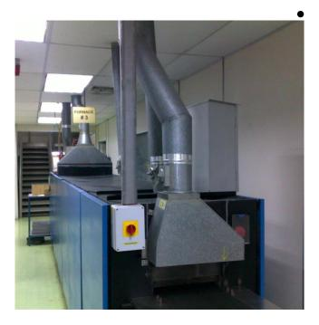
Connect local exhaust ventilation (LEV) at the source of the emission. There should be a sufficient airflow to capture the dust or vapor before it disperses in the workplace. For dust, airflows greater than 1 m/s will generally be needed and for vapours, airflows greater than 0.5 m/s. The airflow should be measured at the origin of the dust or vapor with an anemometer. Provide an easy way of checking that the LEV is working such as a ribbon strip attached to the output side.
