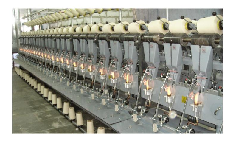
Singeing: the burning-off of loose fibers not firmly bound into the yarn and/or fabric structure.
