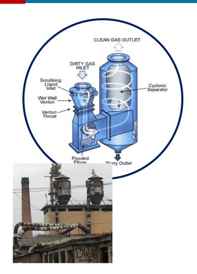
The trapped contaminants are conveyed by ducts to a collector (cyclone, filter house, scrubbers or electrostatic precipitators) where they are removed before the air is discharged into the outside environment.
