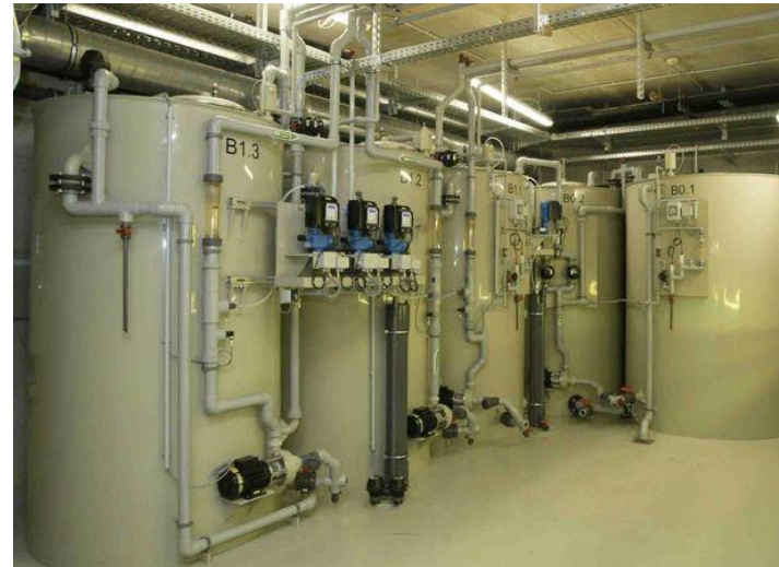
Photo Fenton reactor (Model: ENVIOLET)
