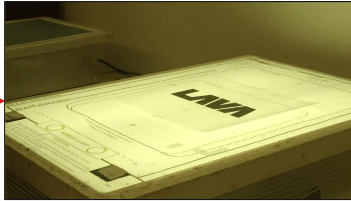
Screen placement and marking
