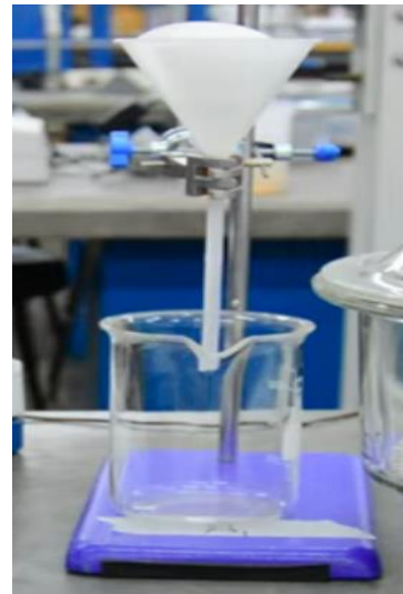
Filter the effluent through filter paper cone
