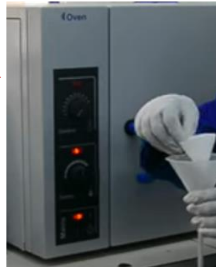
Dry it in the oven @ 104°C for minimum one hour
