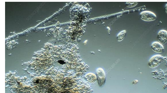
Micro-organisms in MLSS as seen in microscope
