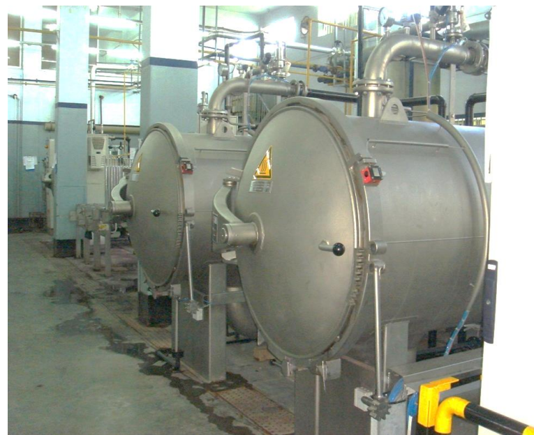
Yarn dyeing in closed vessels
