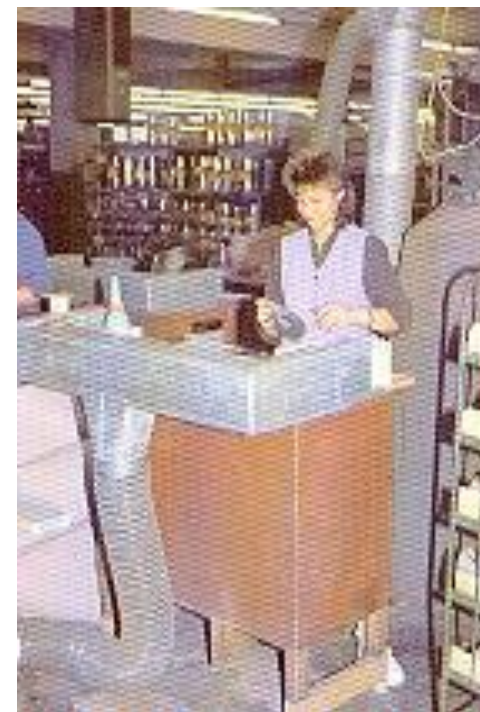
Glue application in shoe factory
