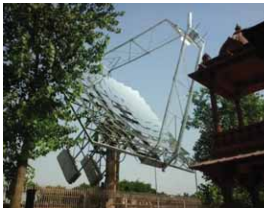
Image no. 3-25: Example of renewable energy application for steam generation at Akshar Dham temple, new Delhi for community cooking
