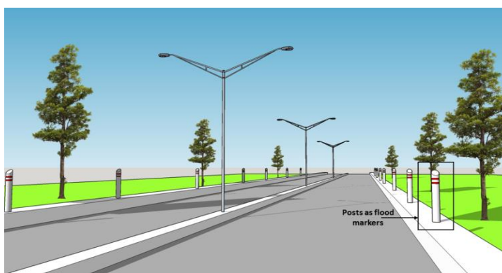
Figure 27: Vertical Posts for Road Safety
