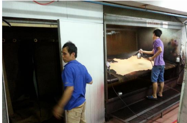
Exhaust system for leather spraying
